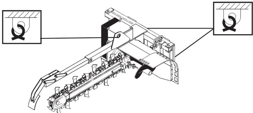
**WARNING!** Verify that all tie down accessories (chains, slings, ropes, shackles and etc.) are capable of maintaining attachment stability during transporting and are attached in such a way to prevent unintended disengagement or shifting of the unit. Failure to do so could result in serious personal injury or death.
