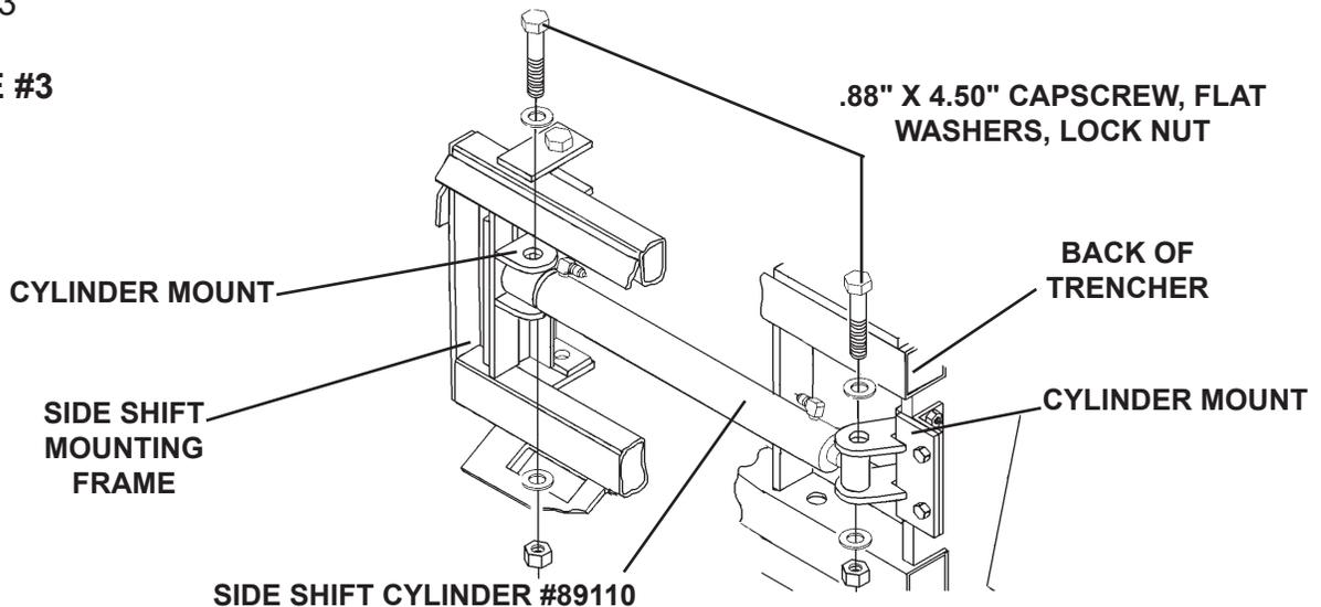
5. If you have hydraulic side shift kit #89279 without a selector valve, installation is complete. If you have hydraulic side shift kit #89412 with selector valve continue with step #6.
