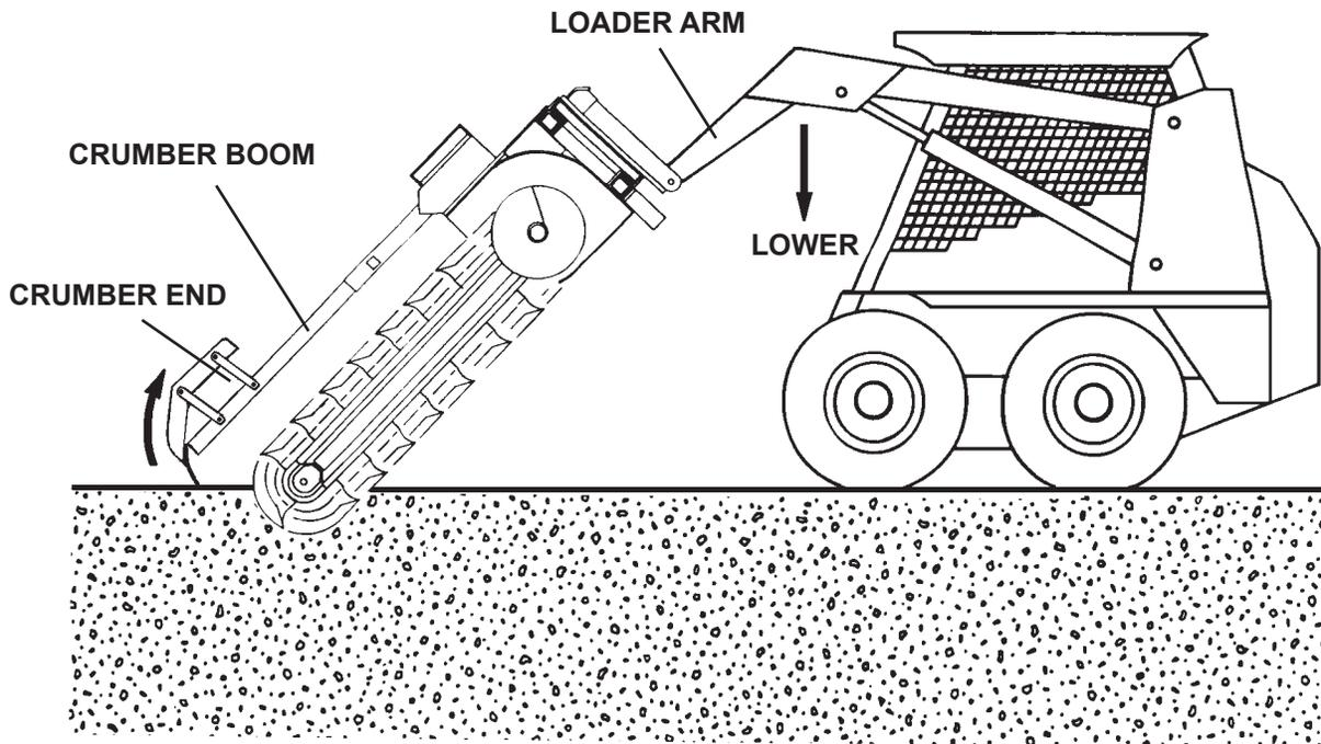
Once the crumber end has "bottomed out", begin slowly creeping the skid steer in reverse while continuing to lower the loader arms. When nearing the required depth, stop lowering and tilt the trencher to a 60° to 65° angle. A 60° - 65° angle works best for general trenching. (See Figure #8)
