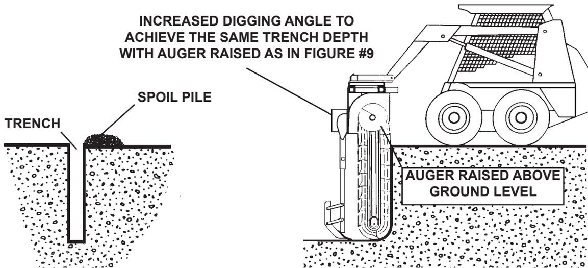
With the desired trench depth reached, advance the skid steer throttle to the desired engine RPM (we suggest full throttle for maximum digging power). Continue creeping the skid steer in reverse. Monitor the skid steer hydraulic oil pressure and temperature gauges as you trench. If hydraulic oil temperature or pressure gets too high, reduce skid steer creeping speed to reduce the load on the auxiliary hydraulic system.
