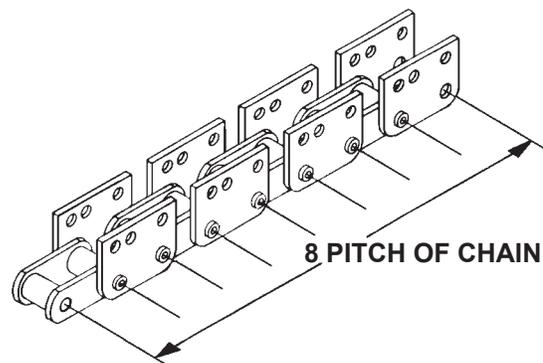
The 625 Trencher has a heavy weight chain with a tensile strength of 50,000 pounds and a pitch of 2.00".
