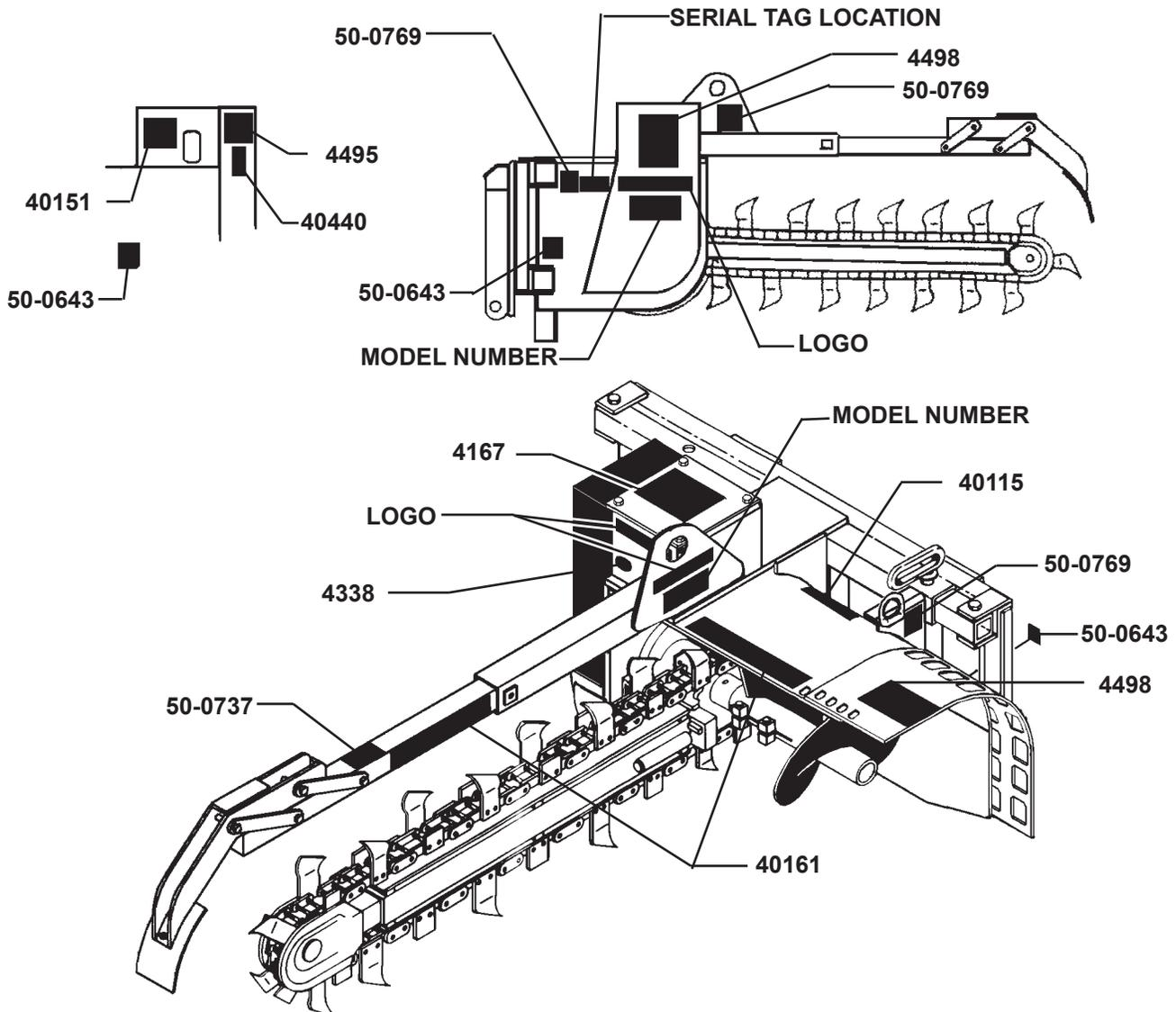
**IMPORTANT:** Keep all safety decals clean and legible. Replace all missing, or damaged safety decals. When replacing parts with safety decals attached, the safety decals must also be replaced.
