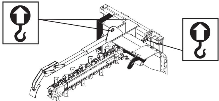
**WARNING!** Use lifting accessories (chains, slings, ropes, shackles and etc.) that are capable of supporting the size and weight of your attachment. Secure all lifting accessories in such a way to prevent unintended disengagement. Failure to do so could result in the attachment falling and causing serious personal injury or death.
