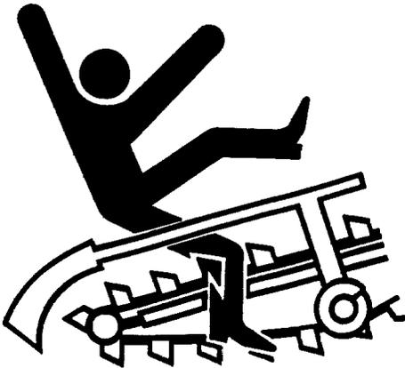
**Stand clear of digging chain and trench. Contact with chain and teeth or cave in of trench wall can cause serious injury or death.**
