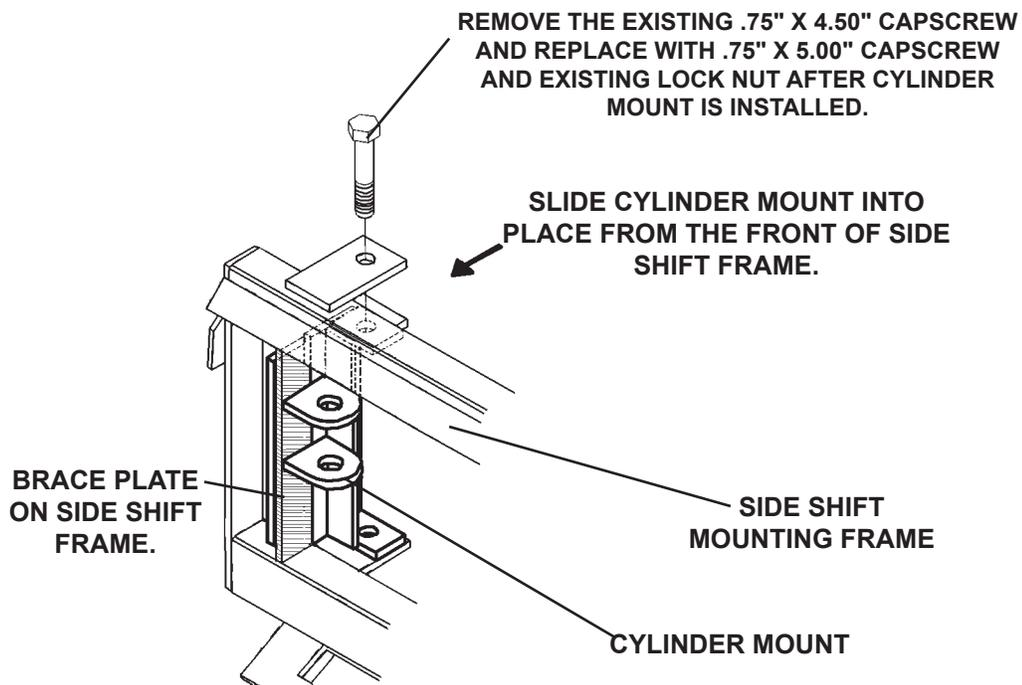
3. Place the remaining cylinder mount on the inside of the .75" plate on the back of the trencher as shown in Figure #2 with the angle mount on the outside of the plate. Align the holes and install the .50" x 2.00" capscrews through the cylinder mount, the trencher and the angle mount while using the .50" x 1.25" capscrews through the cylinder mount and the angle mount. Install the flat washers and lock nuts provided. See Figure #2.
