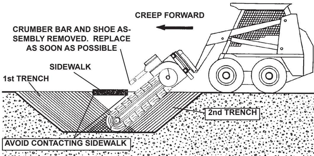
Reinstall the crumber bar and crumber shoe assembly immediately. Some spoil will be left in the trench since the crumber was removed during the operation.
