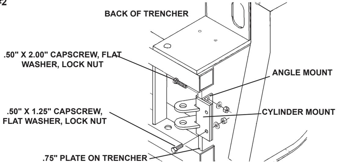
4. Install the side shift cylinder assembly #89110 into the cylinder mounts and secure in place using the .88" x 4.50" cap screw, flat washers and lock nut provided. See Figure #3
