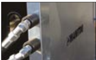
(1) Fully enclosed hydraulic components & connector sockets
