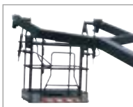
Pendular platform allows work under-bridges
