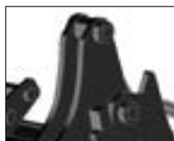
Mechanical rotation stops
