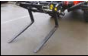
Floating forks with levelling
