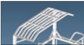
FOPS roof for a maximum protection
