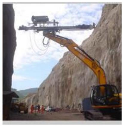
High reach – to be used in development quarry, civil construction and production
