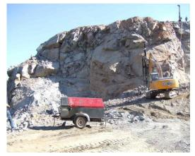
Hydraulic Driven Compressor In this case use the hydraulic System from excavator, but should have a bigger excavator (at least 30 ton)
