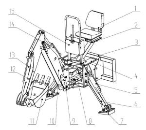
1. seat 2. seat frame 3. hitch frame 4. hitch frame 5. leg cylinder 6.
