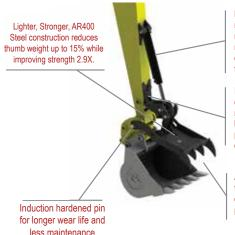
Dual cushioned cylinders reduce machine jarring on extend and retract cycles leading to lower maintenance and smoother operation. Increased clamping force from larger 5" cylinder.
