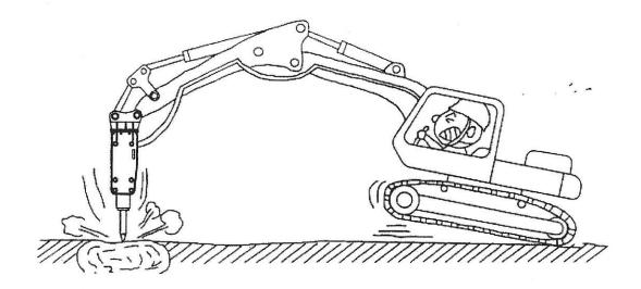
• Apply same direction of boom force in line with the rod and place the rod in the rock with hammering surface as vertical as possible. If hammering surface is oblique, the rod may slip during hammering. This causes the rod to seize and to be broken and piston to be damaged. When breaking, fully stabilize the rod first and then select the point of a rock on which hammering can be performed in a stable condition
