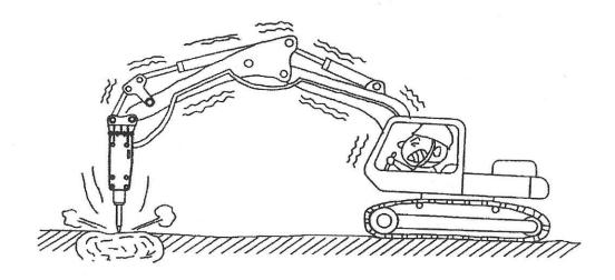
• On the contrary, when position is excessive enough to break rocks with front of the base machine raised, the machine may suddenly tilt forward at the moment rocks are broken. Then, the breaker body or the end of bracket may violently hit against rocks and result in damage.
