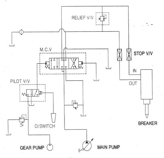
Recommended circuit relief setting pressure and back pressure
