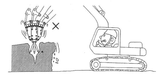
Do not do breaking operation at the stroke end of the carrier cylinder.
